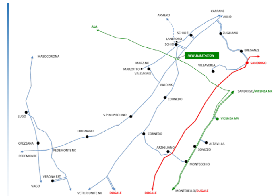
220kV Schio substation and grid upgrade – Category: “Quality, security and resiliency of electricity transportation Infrastructure”
